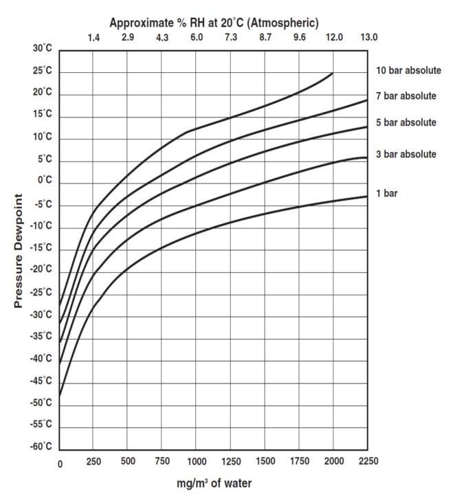
To establish pressure dewpoint, take the point where the water tube reading in mg/m<sup>3</sup> intersects system pressure and read off pressure dewpoint from vertical scale.
