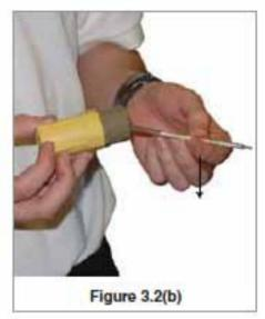
3. Insert the detection tube in the relevant tube receptor in the AIRQUAL-1. Refer to the legend on the top left of the back plate (11. Fig. 2, page 7).
